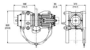
Disc/Pad Braking Minimum Caliper Force Pressure for Full Air Gap kN (lb) Retraction bar (psi) Type mm (in) VS230 4 (0.08) 185 (41590) 180 (2611) VS205 4 (0.08) 165 (37093) 163 (2364) VS190 4 (0.08) 153 (34396) 154 (2234) VS175 4 (0.08) 141 (31698) 144 (2089) VS155 4 (0.08) 125 (28101) 131 (1900) VS137 4 (0.08) 111 (24954) 108 (1566) VS100 4 (0.08) 81 (18210) 84 (1218)
