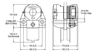
The Twiflex T40 disc brake caliper is split caliper design suitable for use with a minimum disc thickness of 20mm (0.79 in). The modules are mounted each side of a central mounting plate of the same thickness as the brake disc. Minimum disc diameter is 300mm (11.81 in).
