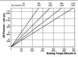
Maximum Pressure 110 bar (1595 psi) Maximum Braking Force = 433kN @ 110 bar (97342.27 lbf @ 1595 psi) Weight of caliper (2 modules) - 580kg (1278.68 lb) Volume displacement per 1mm stroke at both pads = 101.5ml (3.43 fl oz)
