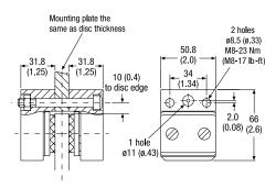
The Twiflex T2 disc brake caliper is split caliper design suitable for use with a minimum disc thickness of 5mm (0.20 in). The modules are mounted each side of a central mounting plate of the same thickness as the brake disc. Minimum disc diameter is 120mm (4.72 in). Alternatively, the brake may be sidemounted with a spacer equal to the disc thickness between the two halves.
