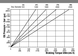
Maximum Pressure 140 bar (2031 psi) Maximum Braking Force = 285kN @ 140 bar (64070.55 lbf @ 2031 psi) Weight of caliper - 287kg (632.73 in) Volume displacement per 1mm stroke at both pads = 51.7ml (1.75 fl oz)
