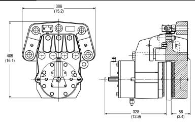
The Twiflex VKSD-FL disc brake caliper comprises a single spring module forming the 'active' side of this floating unit and is available for use where space is limited or to accommodate axial disc float of  $\pm 6$ mm (0.24 in).
