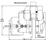
The Twiflex VCS-FL disc brake caliper comprises a single spring module forming the 'active' side of this floating unit and is available for use where space is limited or to accommodate axial disc float of ±6mm (0.24 in).
