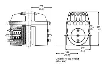
disc, but should ideally be mounted horizontally (i.e. at the 3 o'clock or 9 o'clock position). A range of brake discs is available from Twiflex (see Disc and Hub Assemblies).
